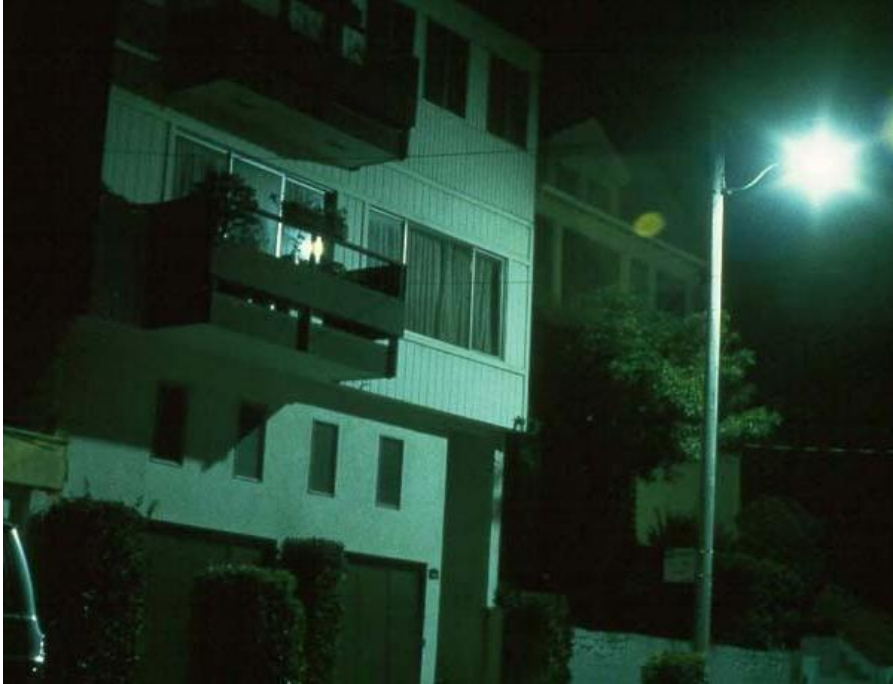
Light trespass above and below horizontal
