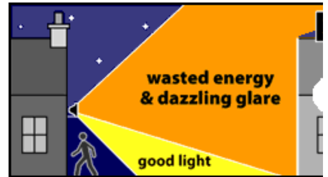
BADLY AIMED 500W HALOGEN FLOODLIGHT
